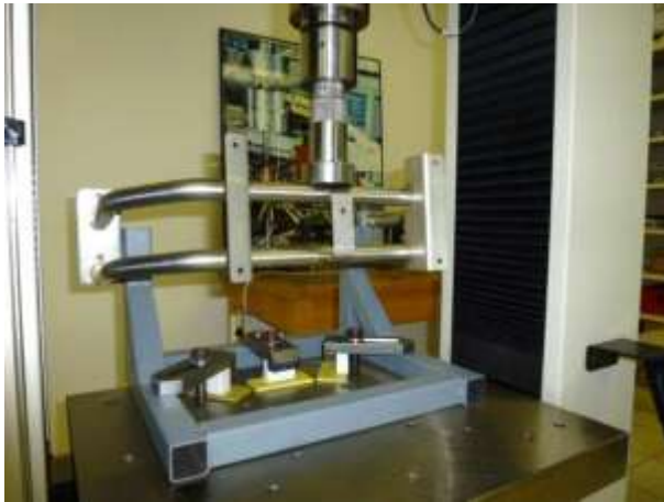
FIG.2A MID-SPAN DOWNWARD LOADING
