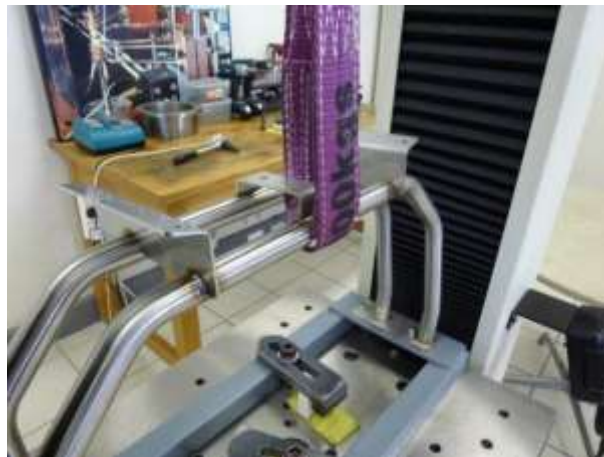
FIG.2C MID-SPAN OUTWARD LOADING
